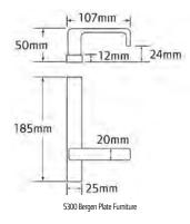
Features & Benefits: 316 marine grade stainless steel. Door thickness: 32mm to 55mm. 75mm screw supplied with external furniture. External screws to suit 56mm to 75mm available on request. Warranty: 30 year mechanical and finish.
